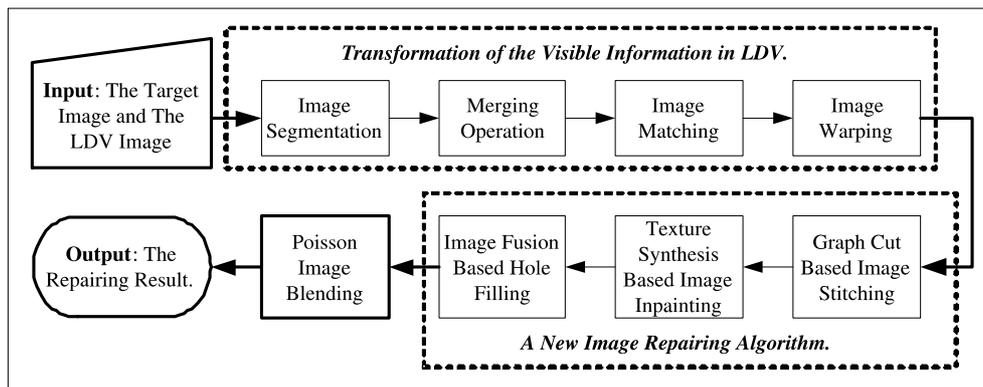
Fig. 1. The pipeline of our method
