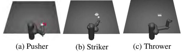
Figure 2: Experimental tasks, Pusher, Striker and Thrower. We change the length of the robotic arm of these tasks to get different environments.
