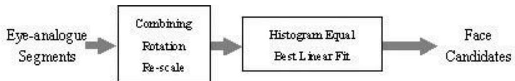
Fig. 5. Block diagram of determining face candidates from eye-analogue segments.
