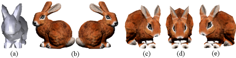
Fig. 6. The rendering effect of mapping two charts of mirrored rabbit onto the Rabbit model
