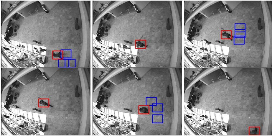
Fig. 6. Browse sequence: The frames 24, 45, 74, 115, 139, 185 are shown. The red boxes are the tracked objects and the blue boxes at 5k + 4 frame are the sampled backgrounds.
