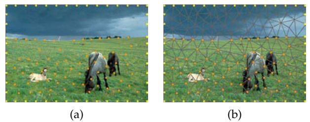
Fig. 2. Mesh generation. (a) Input image with boundary (the yellow dots) and feature points (orange ones) evenly distributed. (b) Delaunay triangulation result. The rest mesh points are added automatically with a distance threshold to maintain mesh uniformity.
