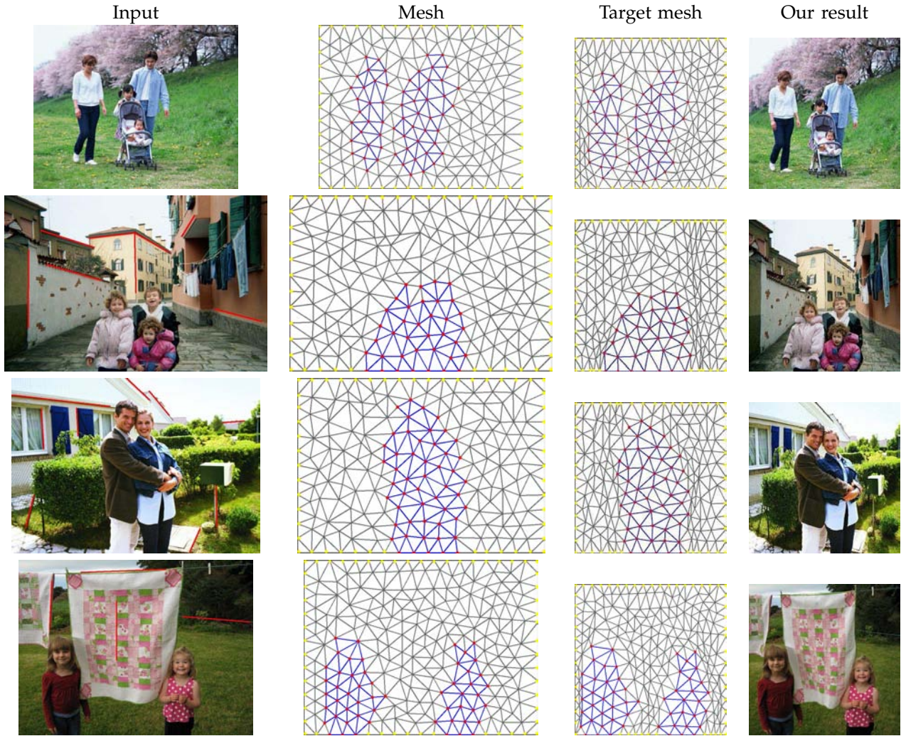
Fig. 8. Our retargeting results. The first column shows the input images with lines detected. The middle two columns are the meshes resulting from triangulation and the target meshes. In the last column, we show our retargeting results.
