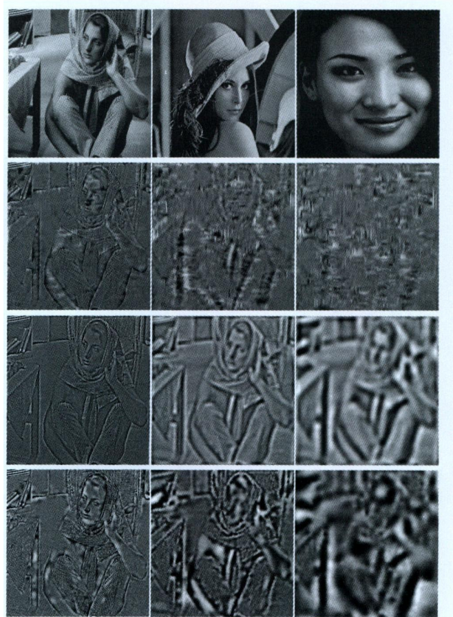
Fig.2. IMFs obtained by decomposing “Barbara” with directional BEMD (the second row), RBF-based interpolation (the third row) and our ALNEMD (the fourth row).
