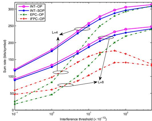
Fig. 4. Sum capacity as a function of the Interference threshold. ( $N_t = 64$ ,  $K = 4$ ,  $K_0 = 2$ .)
