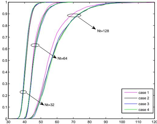
Fig. 8. CDF of the number of Newton iterations required for convergence over 1000 channel realizations. ( $K = 4$ ,  $K_0 = 2$ ,  $P_T = 1W$ .  $\gamma_1 : \gamma_2 = 1 : 1$  (case 1),  $\gamma_1 : \gamma_2 = 1 : 2$  (case 2),  $\gamma_1 : \gamma_2 = 1 : 3$  (case 3),  $\gamma_1 : \gamma_2 = 1 : 4$  (case 4).)
