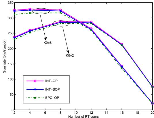
Fig. 5. Sum capacity as a function of number of RT users. ( $N_t = 64$ ,  $L = 2$ ,  $R_k^{req} = 20\text{bit/symbol}$ .)
